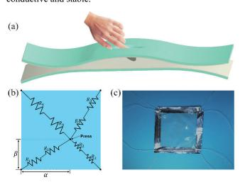
Fig.1: (a) The schematic and working mechanisms of the location sensor; The circuit schematic (b) and real photo (c) of the device.
