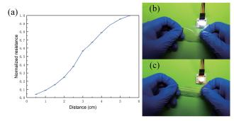
Fig.4: (a) The normalized resistances as a function of distance; The conductivity of the PDMS/AgNWs film under the (b) released and (c) stretched condition.
